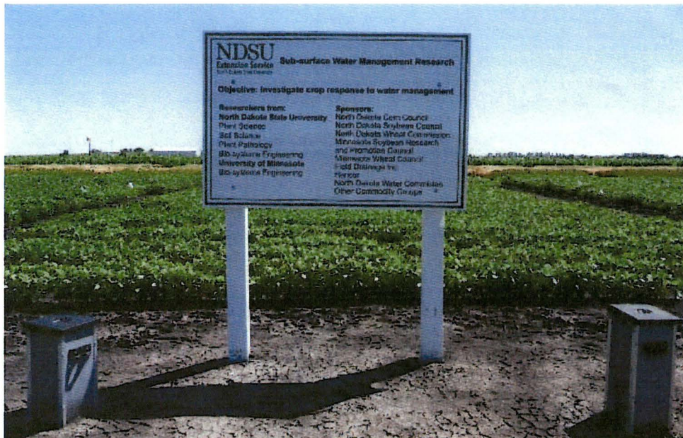
NDSU tile drainage research plots. Note the water level control boxes.
