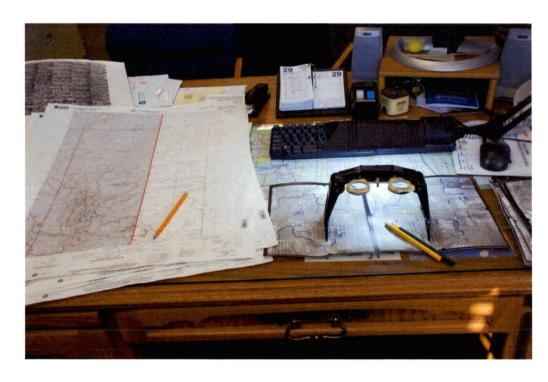
Photograph above: Geologic contacts are identified through the stereoscopes, traced on the photos with grease pencil, the lines are transferred to the quadrangles, and the contacts are checked for accuracy in the field. On the right: Landslide map of the Croff Quadrangle. The landslides are mapped in pink.
