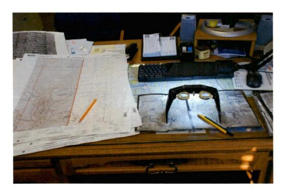
Photograph above: Geologic contacts are identified through the stereoscopes, traced on the photos with grease pencil, the lines are transferred to the quadrangles, and the contacts are checked for accuracy in the field. On the right: Landslide map of the Croff Quadrangle. The landslides are mapped in pink.
