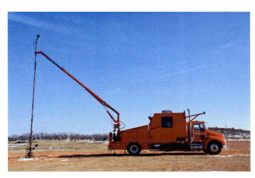
Photograph above: Temperature logging a 10,000 foot well in Mountrail County. Graph on the right: Temperature profile of the Sivertson 29-23R1 in McKenzie County.
