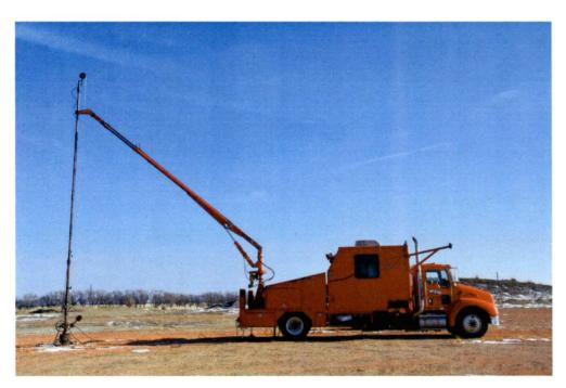
Photograph above: Temperature logging a 10,000 foot well in Mountrail County. Graph on the right: Temperature profile of the Sivertson 29-23R1 in McKenzie County.
