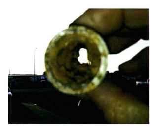
Water sedimentation in pipes.
