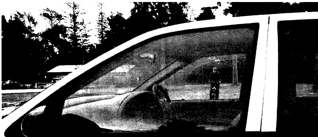
Figure 2.1 View of a cyclist through three front side windows: no tint film and minimal reflection 1
