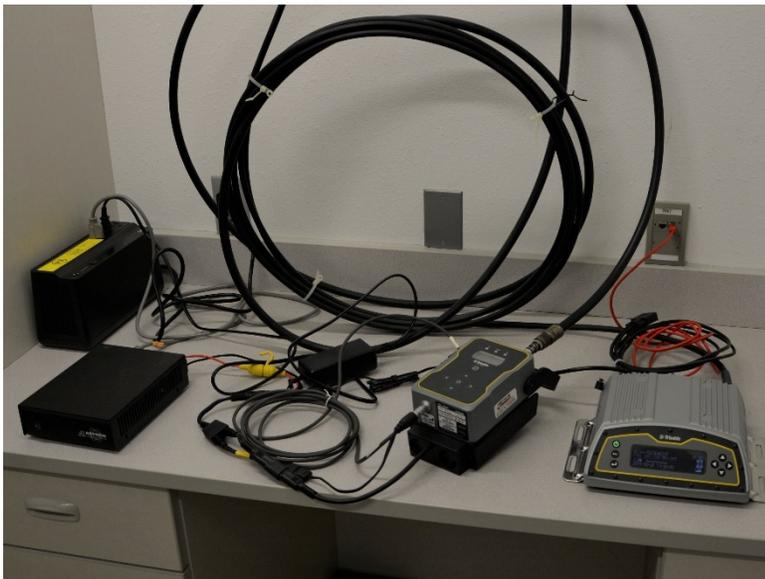
*GPS base station items from left to right: battery backup, ac/dc converter, Trimble TDL 450H GPS data radio, and the new Trimble Alloy GPS receiver.*
