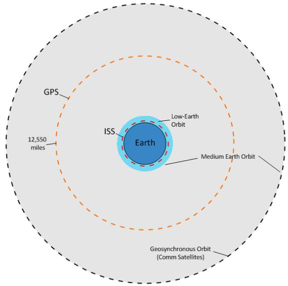
*Left: A schematic of a GPS survey. Right: The GPS base station receives positional signals from two of the main GPS satellite constellations which fly in Medium Earth Orbit, the U.S. GPS satellite constellation (32 satellites) which orbits the Earth twice per day and at an altitude of approximately 12,550 miles, and the Russian GLONASS satellite constellation (24 satellites) which orbit the Earth at an altitude of approximately 11,868 miles.*
