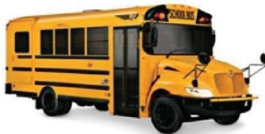
**Type C:** A Type “C” school bus is constructed utilizing a chassis with a hood and front fender assembly. The entrance door is behind the front wheels; also known as a *conventional school bus*. This type also includes cutaway truck chassis or truck chassis with cab with or without a left side door and a GVWR greater than 21,500 pounds.
