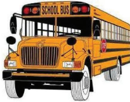
**Type D:** A Type “D” school bus is constructed utilizing a stripped chassis. The entrance door is ahead of the front wheels; also known as *rear or front engine transit style school buses*.
