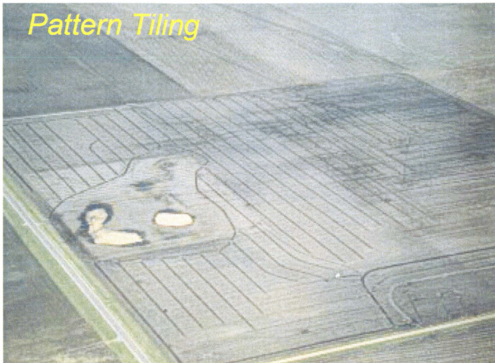
Figure 1. Aerial view of pattern tile drainage in the Dakotas.
