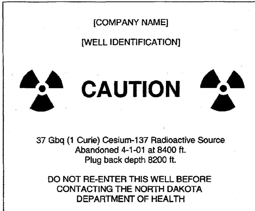
**The size of the plaque should be convenient for use on active or inactive wells, e.g., a 17-centimeter (7 inch) square. Letter size or the word "CAUTION" should be approximately twice the size of the rest of the information.**
